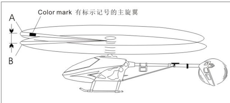
Incorrect tracking may cause vibrations. Please repeat adjusting the tracking to make sure the rotor is correctly aligned. After tracking adjustment, please check the pitch angle is approx. +5° when hovering.
